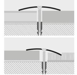
1. Choose the suitable profile and cut it to the necessary length.
