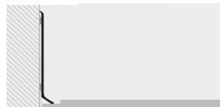
UTILIZZARE PROBAND FIX PER IL FISSAGGIO A PARETE DEL PROFILO NELLA VERSIONE SENZA ADESIVO
