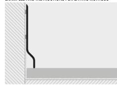
1. Choose the "SKIRTING" in the required the colour. 2. Lay the "SKIRTING" using quick-setting acrylic silicone, mastic or bostik, suitable for gluing flexible PVC onto mortar-plaster-accessorised walls, etc. or fix with screws/nails.
