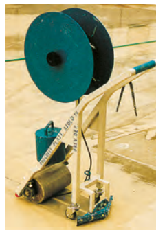
GROUT DRAGGER FOR MORE CONTROLLED LAYING
