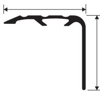
**ANODIZED ALUMINIUM** (6 anod. alum. finishes of which 3 on demand) thermo packed - bar length 2,7 lm - pack. 20 Pcs - 54 lm
