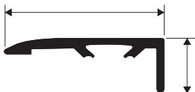
**ANODIZED ALUMINIUM** (6 anod. alum. finishes of which 3 on demand) thermo packed - bar length 2,7 lm - pack. 40 Pcs - 108 lm
