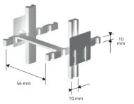
With the **DOPPY** type spacer with double slot, two  $\emptyset$  4 to 8 mm mesh reinforcements may be kept simultaneously at the same distance from the formwork.
