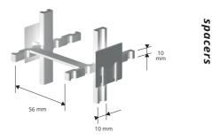
With the **DOPPY** type spacer with double slot, two  $\emptyset$  4 to 8 mm mesh reinforcements may be kept simultaneously at the same distance from the formwork.
