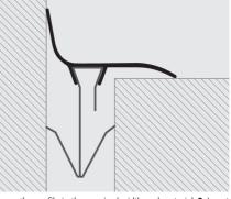
1. Choose the profile in the required width and material. 2. Insert the fixing clips into the relative groove (5 Pcs. for wall applications -10 Pcs. for floor applications). 3. Insert/Lay the PROPLATE FIX in the existing void, applying uniform pressure or using a plastic hammer, thereby creating a perfect joint cover. The same method is used for laying the corner profile.
