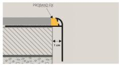
1. Choose "PROTERRACE PCJ" according to the tile thickness and desired colour. 2. Fix the external corners to the screed with nails taking care to separate them at least 1 cm from it. 3. Cut "PROTERRACE PCJ" to the desired length. Lay the profile and fix it with nails. Connect it with the corners using the junctions. 4. Apply the desired waterproofing system. 5. Lay the tiles, leaving about 5 mm between tiles and profile. 6. Seal the space between tiles and profile with **PROBAND FIX (PRBEX)**.
