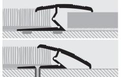
1. Cut the profile to the necessary length. 2. Fix the "PROMOQUETTE GIN" to the floor using screws/nails or two-sided adhesive tape. 3. Lay the required floor, inserting the carpeting, PVC, linoleum, ceramic tile or wood under the upper curved part. **4.** Apply pressure evenly on the edges of the profile until they close and secure the flooring on both sides.
