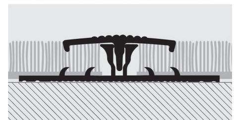
1. Cut the profile to the necessary length. 2. Fix the punched/notched base to the floor using screws/nails or two-sided adhesive tape. 3. Lay the carpeting by gluing or holding under tension. 4. With the help of a wooden tapping block and a hammer, apply pressure evenly over the whole of the top profile until it clicks into the base, thereby securing the carpeting on both sides.
