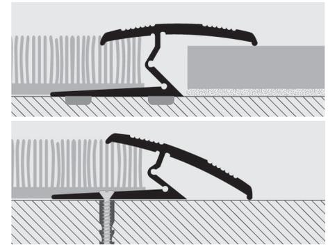
1. Cut the profile to the necessary length. 2. Fix the "PROMOQUETTE GIN" to the floor using screws/nails or two-sided adhesive tape. 3. Lay the required floor, inserting the carpeting, PVC, linoleum, ceramic tile or wood under the upper curved part. 4. Apply pressure evenly on the edges of the profile until they close and secure the flooring on both sides.
