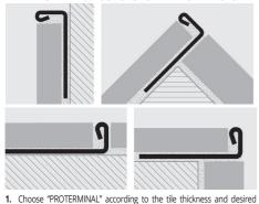
SATIN FINISH STAINLESS STEEL AISI 304/1.4301-V2A with protective film bar length 2,7 lm - pack. 40 Pcs - 108 lm - 10/10 mm
